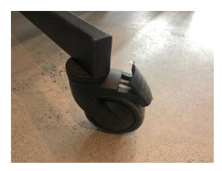
This image shows a castor with the brake engaged. To disengange the brake, push the top of the plastic lever backwards and downwards until it releases and springs back to the disengaged state shown in the image above.
