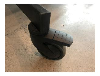
This image shows a castor with the brake disengaged. To engange the brake, push the tip of the plastic lever down with your foot until it clicks. The image below shows how far you must push the lever for it to engage.
